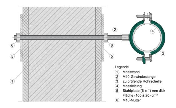
Depending on the equipment of the pipe clamp, fastening can also be carried out with an M - 10 threaded rod with a suitable nut.
